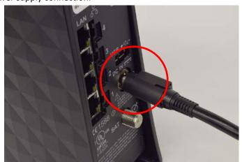
Figure 4: Incorrect power cord connection
