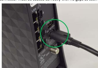
Figure 3: Correct power cord connection
