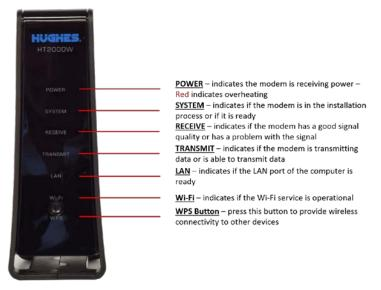
Figure 5: HT2000W LEDs
